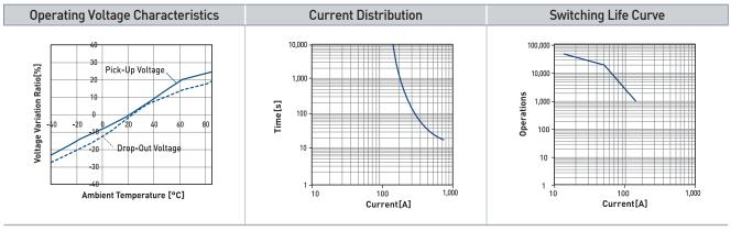
Note : I-T curve at ambient temperature of 23  $^{\circ}\!\text{C}$
