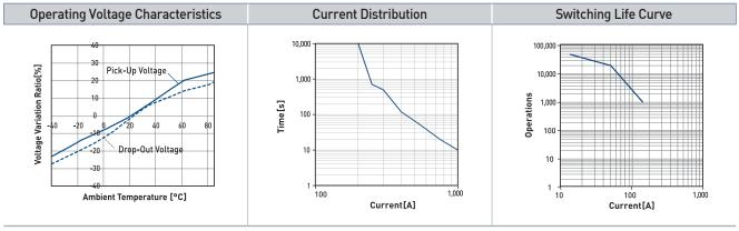
Note : I-T curve at ambient temperature of 23  $^{\circ}\!\!\mathrm{C}$
