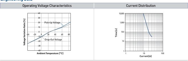
Note: I-T curve at ambient temperature of 23°C
