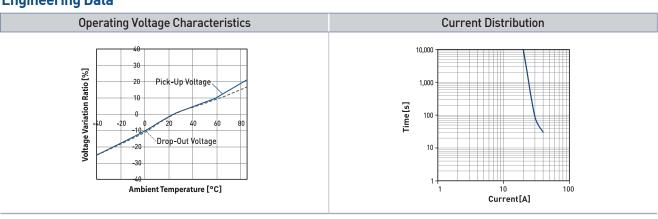
Note : I-T curve at ambient temperature of 23℃
