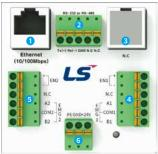
**6** Power terminal block DC 24 V input terminal block
