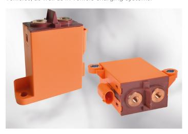
Based on the proven technology of TE's EVC 250 contactor, the EVC 175 contactor features a continuous current of 175 A and a short circuit capability of 5kA, meeting medium power performance requirements. This high voltage contactor does not require inert gas filling or hermetic sealing of the contact chamber, ensuring safe disconnection of overcurrents up to 1,500 A, even at altitudes of 5,500 meters above sea level.
