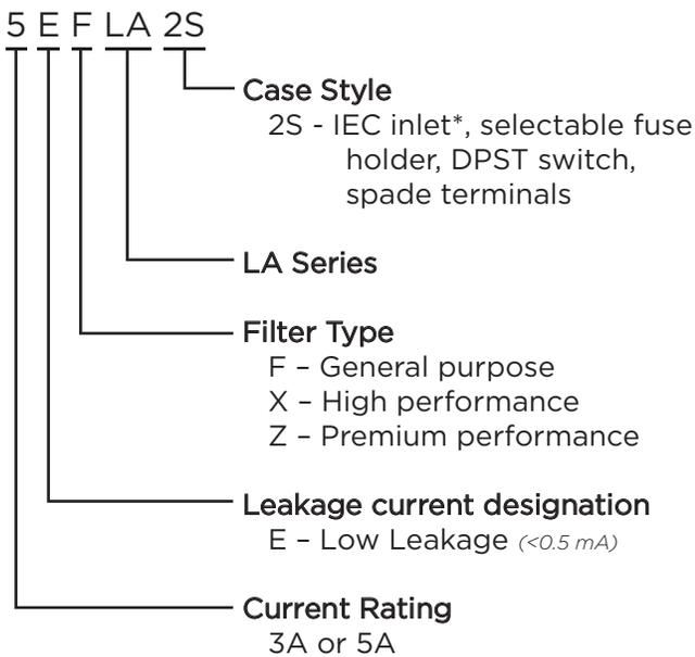
\*IEC 60320-1 C14 inlet mates with C13 connector
