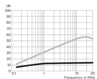
**Minimum Insertion Loss** Measured in closed 50 Ohm system
