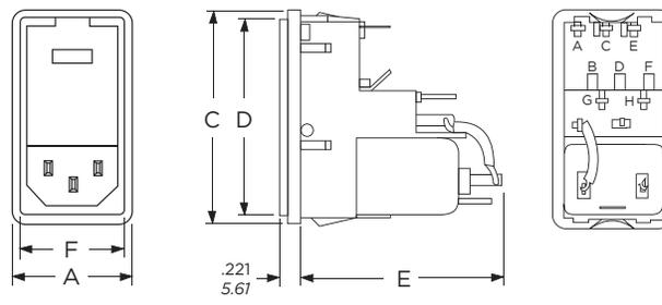
Non-switched model shown, for switched detail refer to flange models
