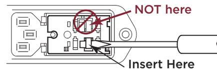
*When the fuse holder is installed in the dual fuse position, it will normally release as soon as the door is opened*
