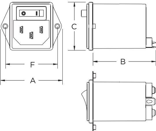
For rear mounted applications only. Maximum panel thickness: .157 [4.0]
