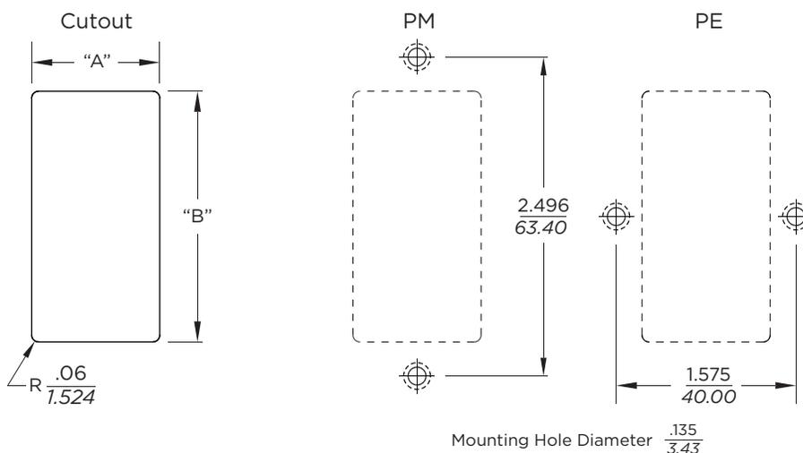
Note: For snap-in applications, the "A" sides must have a .020 [508] radius on the installation side. Dimensions are for front mount applications. Rear mount dimensions should be determined based on customer's application parameters. Snap-in models allow for front mounting only. Not recommended for use in plastic panels.
