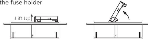
4. When the fuse holder is installed in the single fuse position, apply the screwdriver as shown and gently lift up. Use screwdriver as shown, do not use fingers
