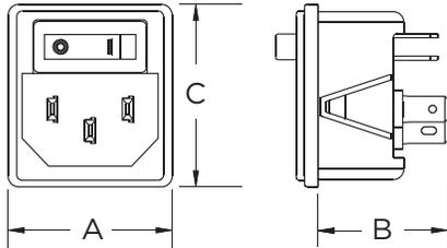
Available for panel thickness .07 - 1.0mm (CU10S1) or 1.2 - 1.5mm CU15S1
