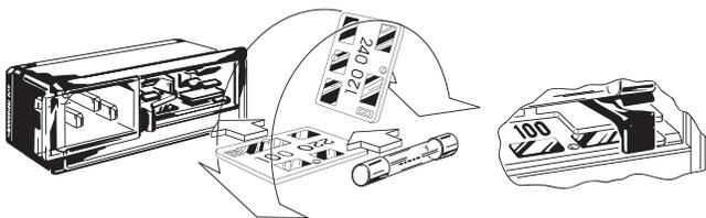
Open cover door and slide fuse-pull lever to left. Select operating voltage by orienting voltage selection card with the desired voltage on top left side. Push card firmly into module slot. Slide fuse-pull lever to right into normal position and re-insert fuse into holders.
