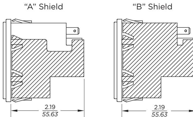
Note: Shields can only be used with filtered models. B shield may not be used with J or C extender
