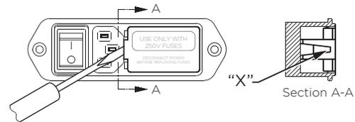
3. Gently lift the entire door UP approximately 1/4" *(minimum)*. Once lifted, the door will pivot on it's hinges to expose the fuse holder
