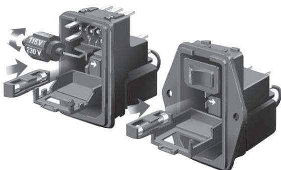
To change selected voltage: disconnect the power cord; open cover using a small blade screwdriver or similar tool; insert the tool into the voltage selection slot and remove wheel from unit; select desired voltage; replace wheel into unit and close cover, making sure the selected voltage appears in connector window.
