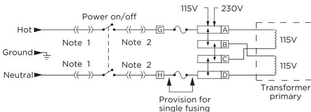
Note 1: Additional jumper wiring is required if a filter or interconnection module is not used.
