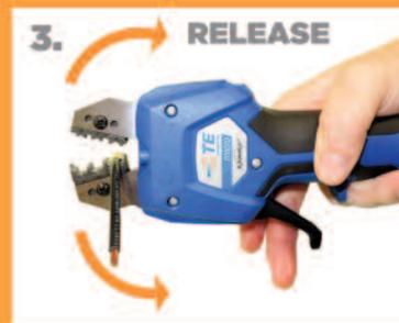
Release trigger and the jaws will open automatically.
