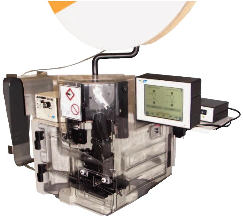
These value-oriented terminators are based on the field-proven AMP-O-LECTRIC Model G terminator. They are the latest in the series of machines for terminating wire using reeled terminals and contacts. The AMP 3K and AMP 5K terminators are designed for customers that require the increased output and quality of a benchtop, semi-automatic machine at a competitive price. Reliability is evident in features like the direct motor drive system and robust construction.
