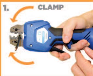
Quick takeup: Pull trigger part way and adjust terminal and wire to the proper position before crimping.
