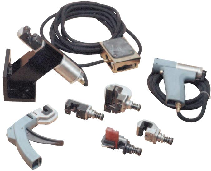
The pistol grip hand tool system uses interchangeable terminating heads to apply a broad range of TE IDC products. The basic tool requires a pistol grip handle assembly and a terminating head; power-assist and bench mount versions are available to suit your specific needs.
