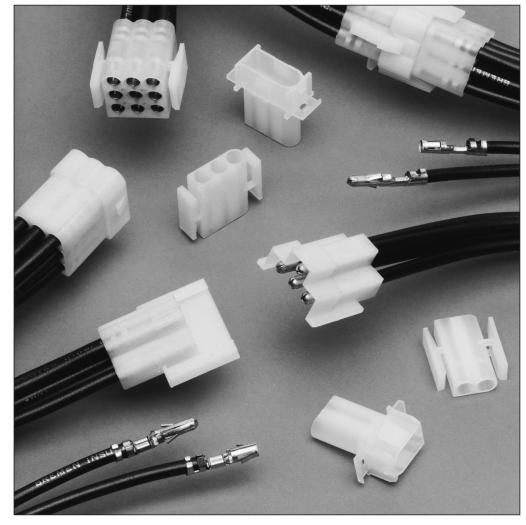
The UL recognized .140 MATE-N-LOK connectors with 3.5 mm diameter pins and sockets, have a 25 A current carrying capacity and are capable of accepting wire with insulation diameters up to 4.5 mm. Both pins and sockets are equipped with dual locking lances, which assure positive contact retention when installed in the housings.
