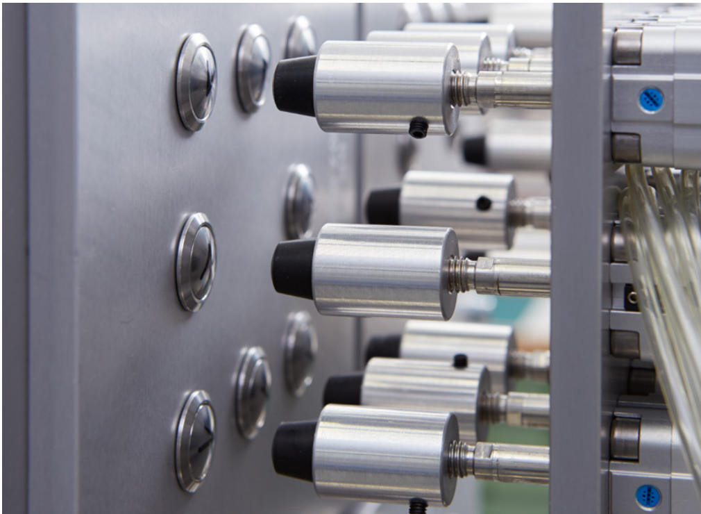
Long term aging test of Series 82. Long service life: More than 1 million cycles of operation.
