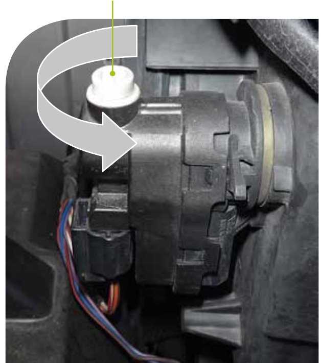
Initial aiming adjustment on the electrical actuator
