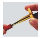
**Step 1:** Snap appropriate size removal tool over the wire.
