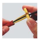
**Step 2:** Hold Jiffy Splice between thumb and forefinger approximately one half inch behind cavity. Slide tool into cavity until resistance is felt and retaining fingers are engaged. Do not twist or insert tool at an angle.
