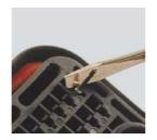
**Step 2:**To remove contacts, gently pull wire backwards, while at the same time releasing the locking finger by moving it away from the contact with a screwdriver.
