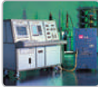
Characteristics Test / VCB Characteristics Test
