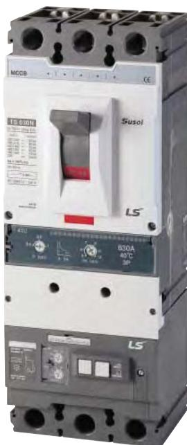
The RCD unit has numerous current and time settings and an override blocking the time settings when set to 30mA. The earth leakage test button tests the electrical and mechanical operation of the device. In order to allow for a dielectric test of the breaker and RCD combination without damaging the electronics, the dielectric plug is placed within the setting area. The RCD unit may be equipped with an alarm switch (FAL) to remotely indicate tripping due to an earth leakage current.
