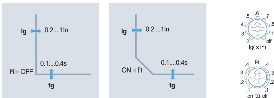
$I_g$  = insulation fault threshold
