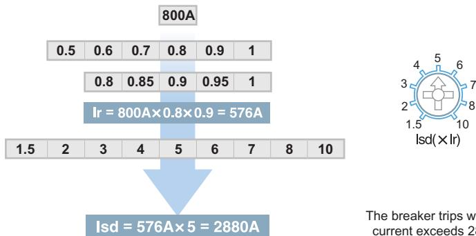
The breaker trips when the current exceeds 2880 A.
