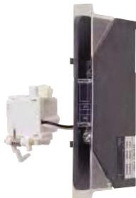
The shunt trip opens the mechanism in response to an externally applied voltage signal. The releases include coil clearing contacts that automatically clear the signal circuit when the mechanism has tripped.
