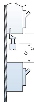
Connection by using a cable terminal or ring terminal
