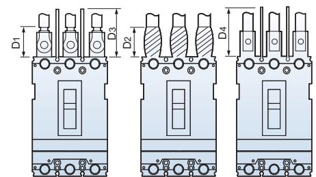
Note) If uninsulated conductors are used for connection, please insulate by taping to the point where the conductors overlap with the insulation barrier or to the root of the circuit breaker.
