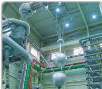
High Voltage Test / Impulse Test
