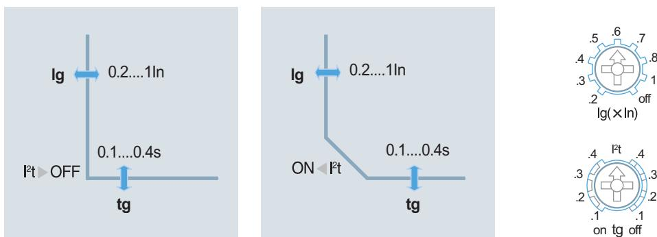
Ig = insulation fault threshold
