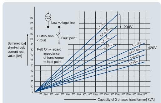
Ref 1) Calculation in the random voltage E Voltage line which is mostly close to E shall be selected to calculate it . i.e. in case of 220V, (200V line value) ÷ 200/220
