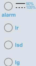
The LED lights and remains lit when the load exceeds 90 % of Ir.
