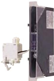
The undervoltage release automatically opens a circuit breaker when voltage drops to a value ranging between 20% to 70% of the line voltage. The operation is instantaneous, and after tripping, the circuit breaker cannot be re-closed again until the voltage returns to 85% of line voltage. Continuously energized, the undervoltage release must be operating before the circuit breaker can be closed. The undervoltage release can be easily installed in the right accessory compartment of the MCCBs.
