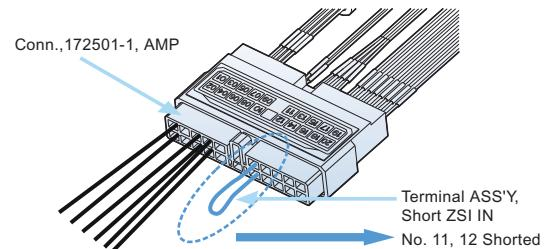
**Caution :** If not using ZSI function of Trip Relay (OCR), please short ZSI INPUT of terminal No.11,12 (ZSI IN +, ZSI IN-) by using the "TERMINAL ASS'Y,SHORT ZSI IN"
