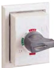
The rotary handle operating mechanism is available in either the direct version or in the extended version on the compartment door. It is always fitted with a compartment door lock and on a request it can be supplied with a key lock in the open position.
