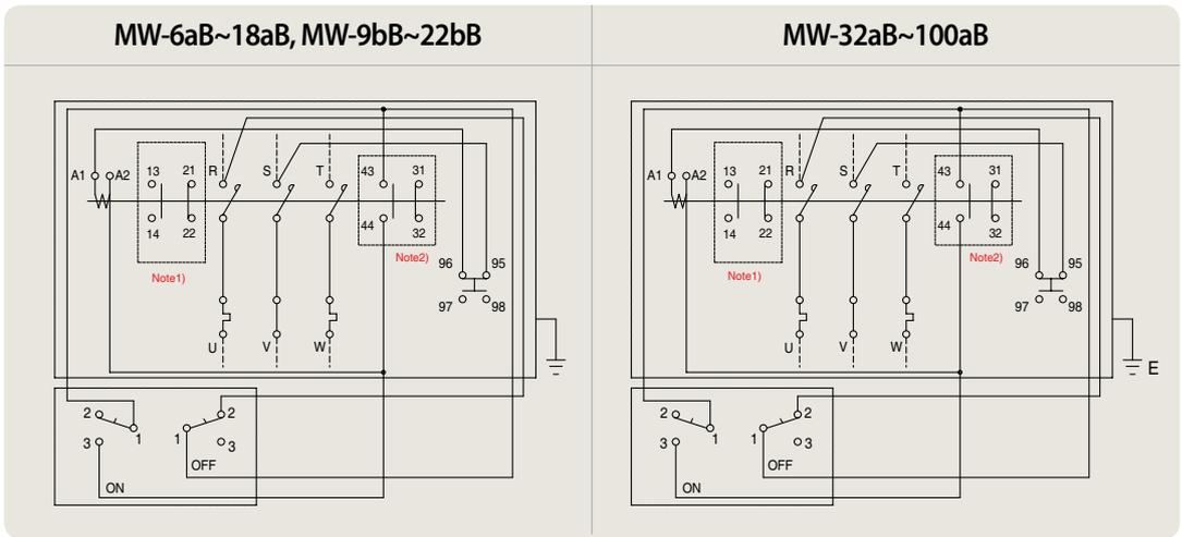
Note 1. In case of adding the auxiliary contact unit(1NO1NC).
