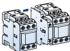
And then install the other contactor on the other side of the interlock unit as shown.
