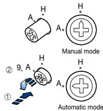
Using a driver the reset mode can be set.
