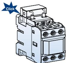
Connect the lead wires to the coil terminals of the contactor first. And then insert the body into the space of the contactor as shown above.
