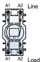
Note) A1(A2) in line side is internally connected to A1(A2) in load side.
