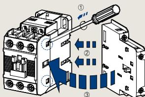
To install side mounting unit remove the indicated part in the fig. first. And then fit each part as shown. To separate push forward and pull.
