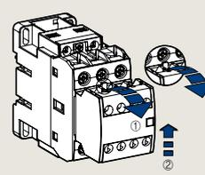
To install front mounting unit fit it on the upper part of the front of the contactor and push it down. To separate pull the lever of the unit and push the unit upward.
