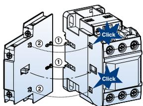
Install the interlock unit on the side of a contactor first. Fit each part as indicated in the fig.
