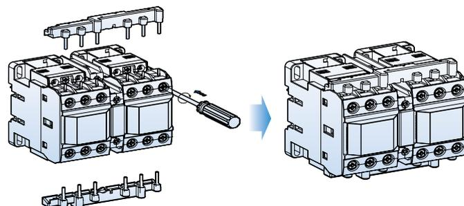
After installing interlock unit wiring kit can be assembled. Wiring kit contains two molded wires - one for line side and the other for load side. - In case of assembling Reversing contactor, please check the R, S, T/U, V, Wmark on the contactor and Wire kit.
