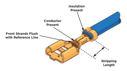
**3.** Crimp Specifications – To ensure a proper crimp for a TE connector or terminal you should be using a TE Connectivity tooling solution that is specifically engineered to the proper Crimp Height, Width and Crimp Geometry of the selected terminal or contact.
