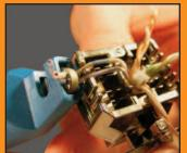
Easily places wire in SL mod jack lacing fixture.
