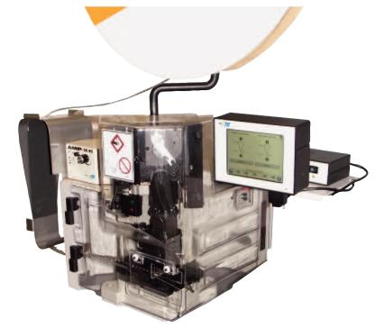
These value-oriented terminators are based on the field-proven AMP-O-LECTRIC Model G terminator. They are the latest in the series of machines for terminating wire using reeled terminals and contacts. The AMP 3K and AMP 5K terminators are designed for customers that require the increased output and quality of a benchtop, semi-automatic machine at a competitive price. Reliability is evident in features like the direct motor drive system and robust construction.
