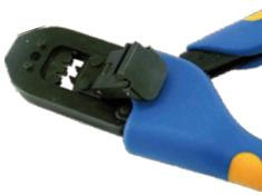
the locator approx. 150 degrees, which provides exact placement of small terminals. After loading, the locator is flipped back into position and the terminal is properly located automatically. Now, with the terminal held in place, the operator can concentrate on proper wire placement and complete the termination process.
