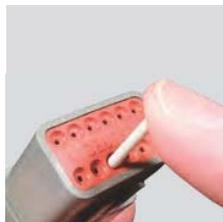
**Step 2:** With perpendicular motion, apply downward pressure to the small diameter end of the sealing plug.
