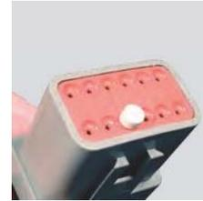
**Step 3:** Apply pressure until sealing plug is forced to stop by contact with rear grommet. Visually inspect the sealing plug to confirm it is flush with cavity opening.
